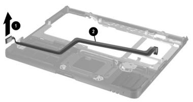
Removing the Bluetooth Wireless Device
